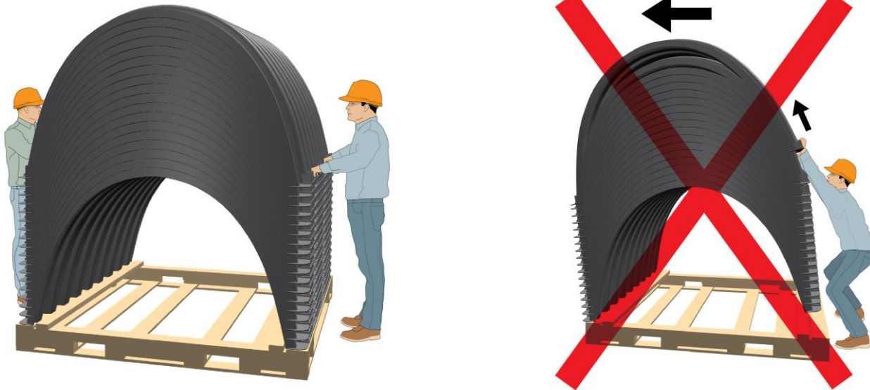
Figure 4 - Chamber Unloading from Pallets
