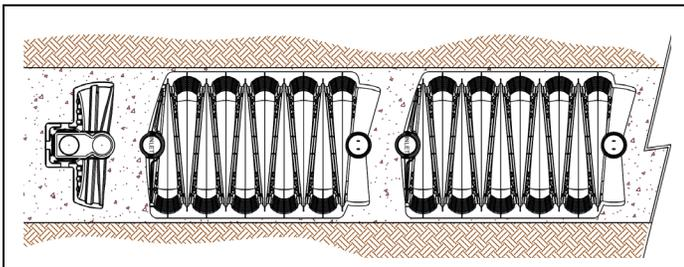
**Step 3:** Place the prepared endcap over the chamber and make sure it is aligned with the header pipe. The endcap will snap into place with locking tabs when pressed down on the chamber.
