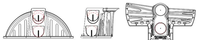
**Step 2:** Install the splash plate by removing the guard from the endcap and inserting the risers of the guard into the channels underneath the endcap footer.
