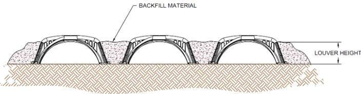
**Step 12:** Compact this soil by walking along the sides of each chamber.
