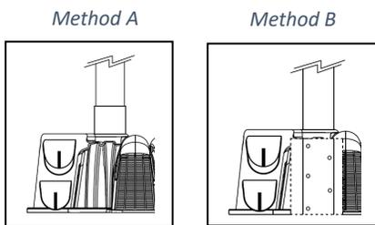
**Step 3:** Secure the pipe using a screw thru the coupler ring.
