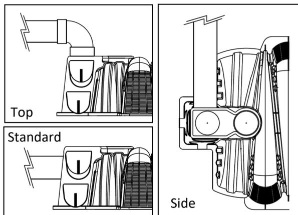
**Step 4:** Insert the inlet pipe into the prepared endcap opening. The pipe should be inserted at least 2”.
