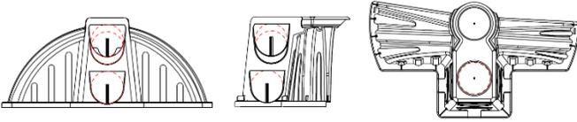
**Step 2:** Install the splash guard by removing the guard from the endcap and inserting the risers of the guard into the channels underneath the endcap footer.
