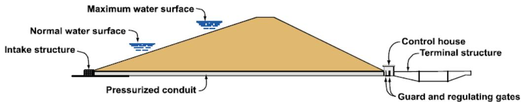
**Figure 1. Pressurized Outlet Works**
