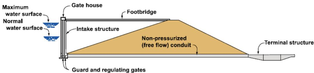
**Figure 2. Non-Pressurized Outlet Works**
