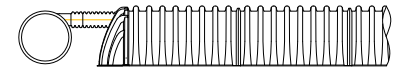
FIGURE 8. HEADER WITH REDUCING STUB AT CROWN INTO TOP OF END CAP WITH HEADER INVERT AT OR BELOW STUB INVERT.
