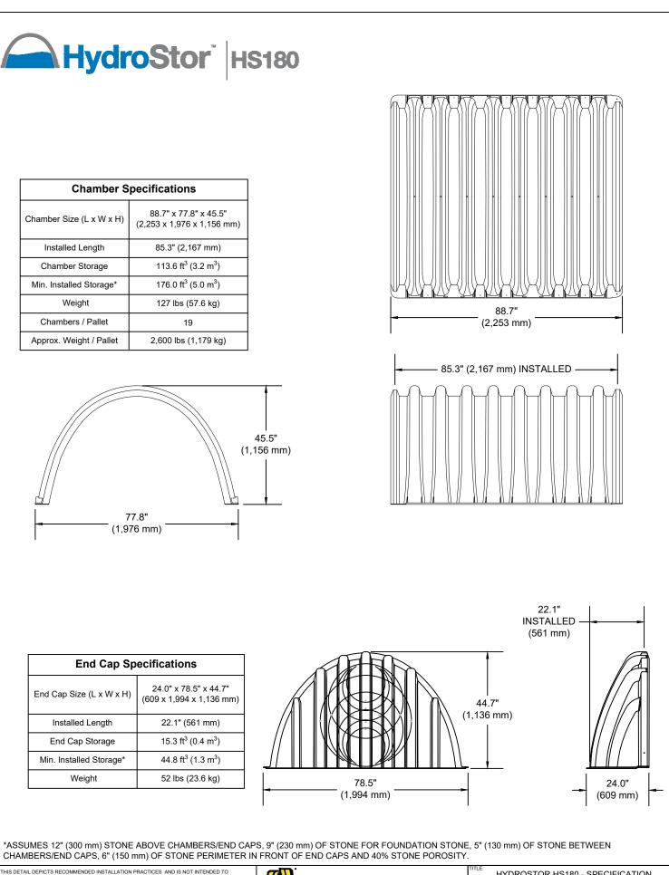
THIS DETAIL DEPICTS RECOMMENDED INSTALLATION PRACTICES AND IS NOT INTENDED TO SUPERSEDE ANY NATIONAL, STATE OR LOCAL SPECIFICATIONS. PRINSCO BEARS NO RESPONSIBILITY FOR ANY ALTERATIONS, REVISION AND/OR DEVIATION FROM THIS STANDARD DETAIL PRINSCO HAS NOT PERFORMED ANY ENGINEERING OR DESIGN SERVICE FOR THIS PROJECT. THE DESIGN ENGINEER SHALL REVEW THESE DETAILS PRIOR TO CONSTRUCTION TO VERIFY SUITABILITY. © PRINSCO, INC.
