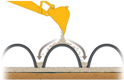
Figure 20 - Backfill Placement with Excavator
