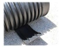
**Step 3:**Set the adjoining pipe or fitting on the coupler and wrap the coupler around
