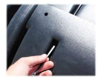
**Step 5:**Thread zip ties through the holes in the middle valleys of each coupler, securing both ends of the coupler together.
