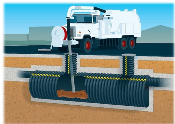
Figure 2: Vacuum Truck with Hose
