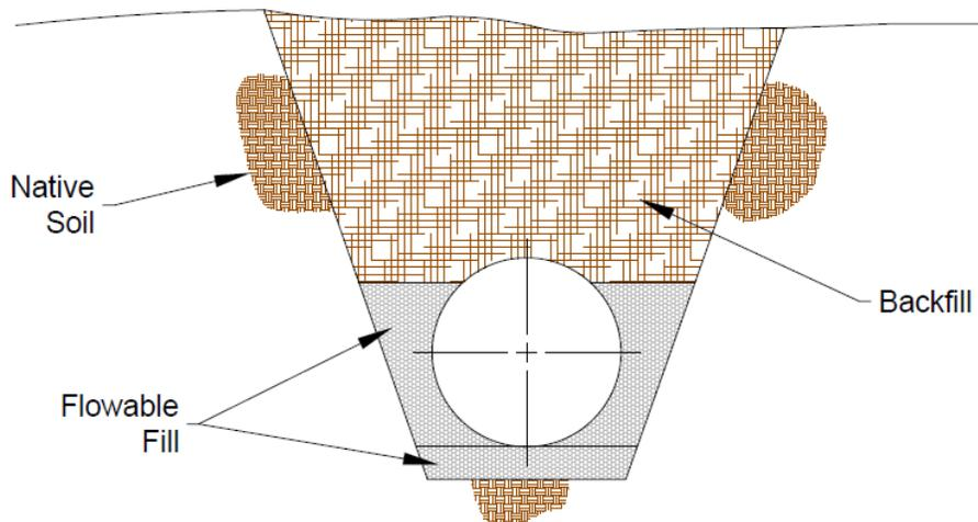
Figure 1: Flowable Fill Backfill
