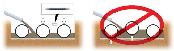
Figure 3: Pipe Anchoring to Prevent Floatation
