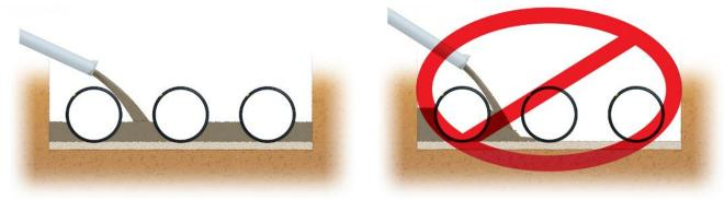
Figure 2: Flowable Fill Placement Recommendation
