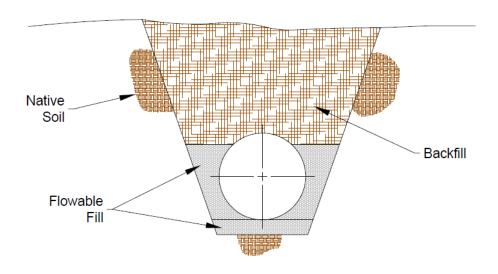
Figure 1: Flowable Fill Backfill
