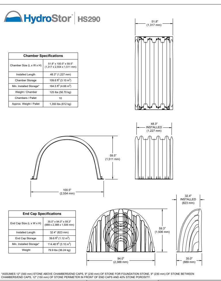
THIS DETAIL DEPICTS RECOMMENDED INSTALLATION PRACTICES AND IS NOT INTENDED TO SUPERSEDE ANY NATIONAL, STATE OR LOCAL SPECIFICATIONS. PRINSCO BEARS NO RESPONSIBILITY FOR ANY ALTERATIONS, REVISION AND/OR DEVIATION FROM THIS STANDARD DETAIL. PRINSCO HAS NOT PERFORMED ANY ENGINEERING OR DESIGN SERVICE FOR THIS PROJECT. THE DESIGN ENGINEER SHALL REVIEW THESE DETAILS PRIOR TO CONSTRUCTION TO VERIFY SUITABILITY. © PRINSCO, INC.
