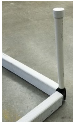
Figure 6: PVC Pipe inserted into port at 90° Elbow
