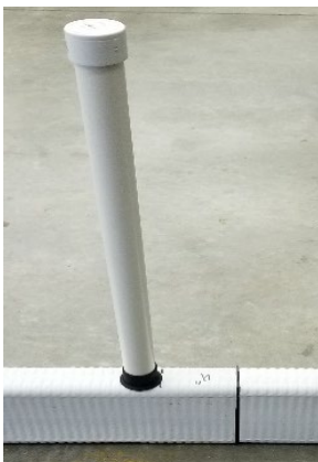
Figure 5: PVC Pipe inserted into port at PFHD stick.
