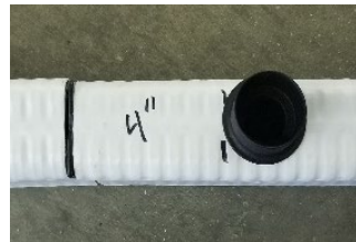
Figure 3: Installed port on PFHD stick.
