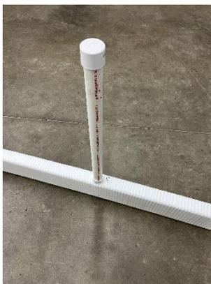
**Figure 5: PVC Pipe inserted into adapter at PFHD stick.**
