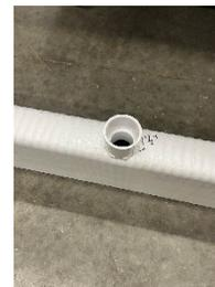
**Figure 3: Installed adapter on PFHD stick.**
