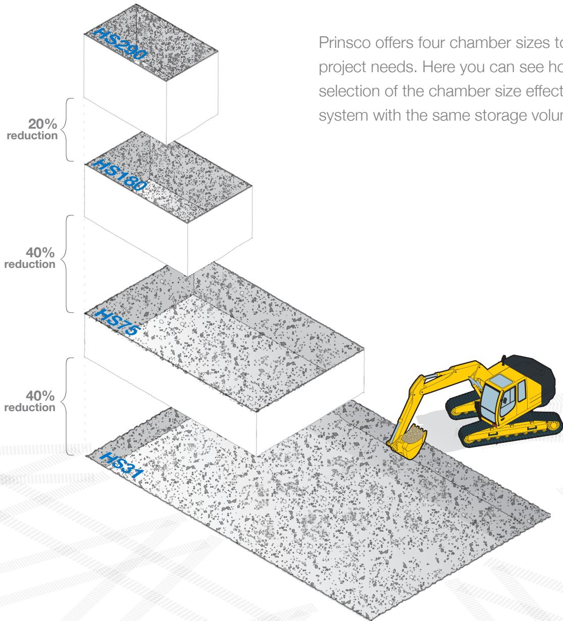
Prinsco offers four chamber sizes to meet various project needs. Here you can see how dramatically the selection of the chamber size effects the footprint of a system with the same storage volume.
