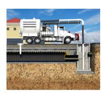
The most common method of cleaning is done by using a vacuum truck. For the sediment row, a high-pressure nozzle with rear facing jets is used to direct the sediment and debris to the inlet control structure where it can then be vacuumed out. Care needs to be taken to ensure damage to the geotextile fabric does not occur when removing sediment and debris.
