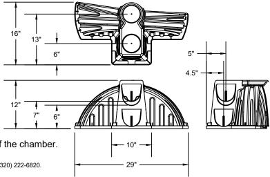
Pro4 36 End Cap can be installed at either end of the chamber.
