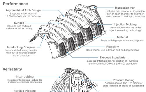
Supports multiple gravity, front, side, and top inletting elevations
