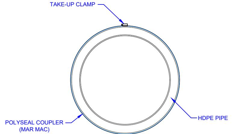
3 POLYSEAL COUPLER SECTION DETAIL
