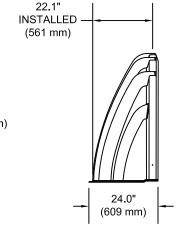
\*ASSUMES 12" (300 mm) STONE ABOVE CHAMBERS/END CAPS, 9" (230 mm) OF STONE FOR FOUNDATION STONE, 5" (130 mm) OF STONE BETWEEN CHAMBERS/END CAPS, 6" (150 mm) OF STONE PERIMETER IN FRONT OF END CAPS AND 40% STONE POROSITY.
