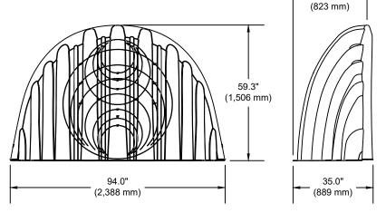
\*ASSUMES 12" (300 mm) STONE ABOVE CHAMBERS/END CAPS, 9" (230 mm) OF STONE FOR FOUNDATION STONE, 9" (230 mm) OF STONE BETWEEN CHAMBERS/END CAPS, 12" (150 mm) OF STONE PERIMETER IN FRONT OF END CAPS AND 40% STONE POROSITY.
