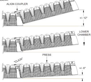
**Note:** Chambers can be disengaged by lifting the end of chamber away from the connection. Multiple disengagements may cause the locking tabs to break. If this occurs, a screw may be used to connect the chambers.
