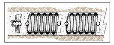
**Step 3**: Place the prepared endcap over the chamber and make sure it is aligned with the header pipe. The endcap will snap into place with locking tabs when pressed down on the chamber.
