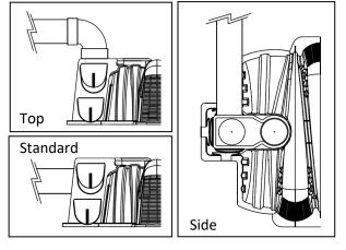
**Step 4**: Insert the inlet pipe into the prepared endcap opening. The pipe should be inserted at least 2 inches.
