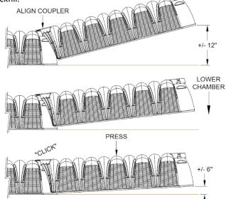
**Note:** Chambers can be disengaged by lifting the end of chamber away from the connection. Multiple disengagements may cause the locking tabs to break. If this occurs, a screw may be used to connect the chambers.
