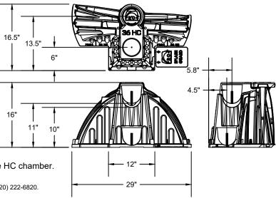
Pro4/36 HC Endcap can be installed at either end of the HC chamber.
