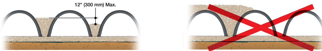
Figure 21 - Embedment Stone Placement
