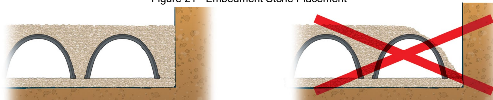
Figure 22 - Perimeter Backfill Placement
