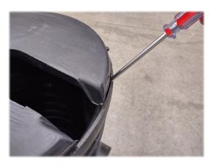
If the lid needs to be removed, use a screwdriver or other prying device and work around the lid in a clockwise fashion.
