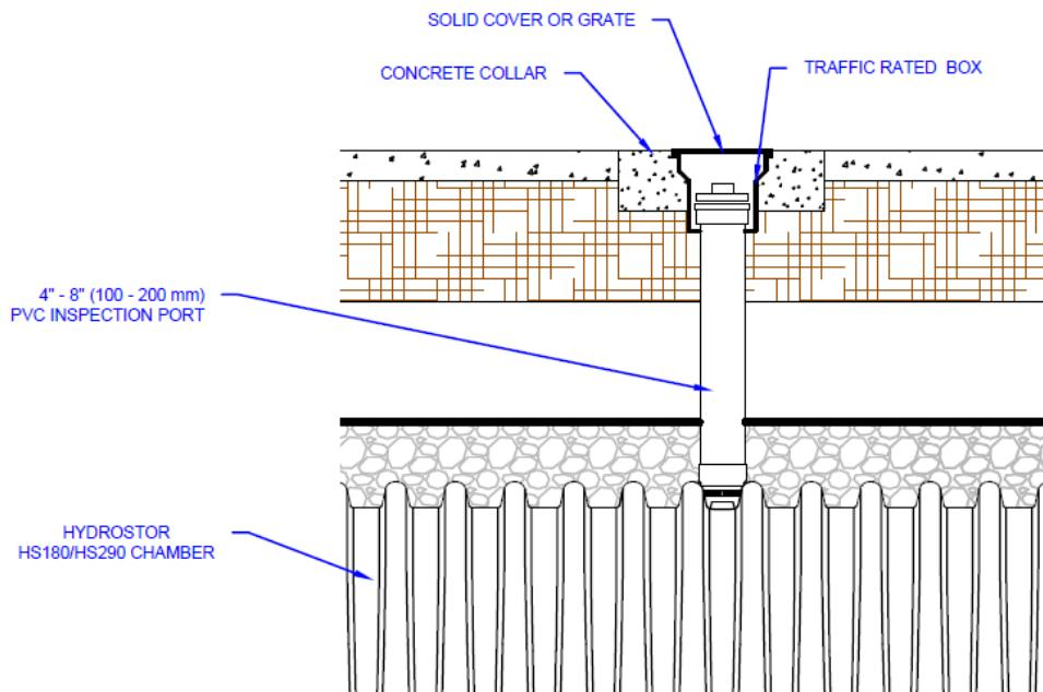
Figure 19 - Inspection Ports for Chamber Sediment Rows
