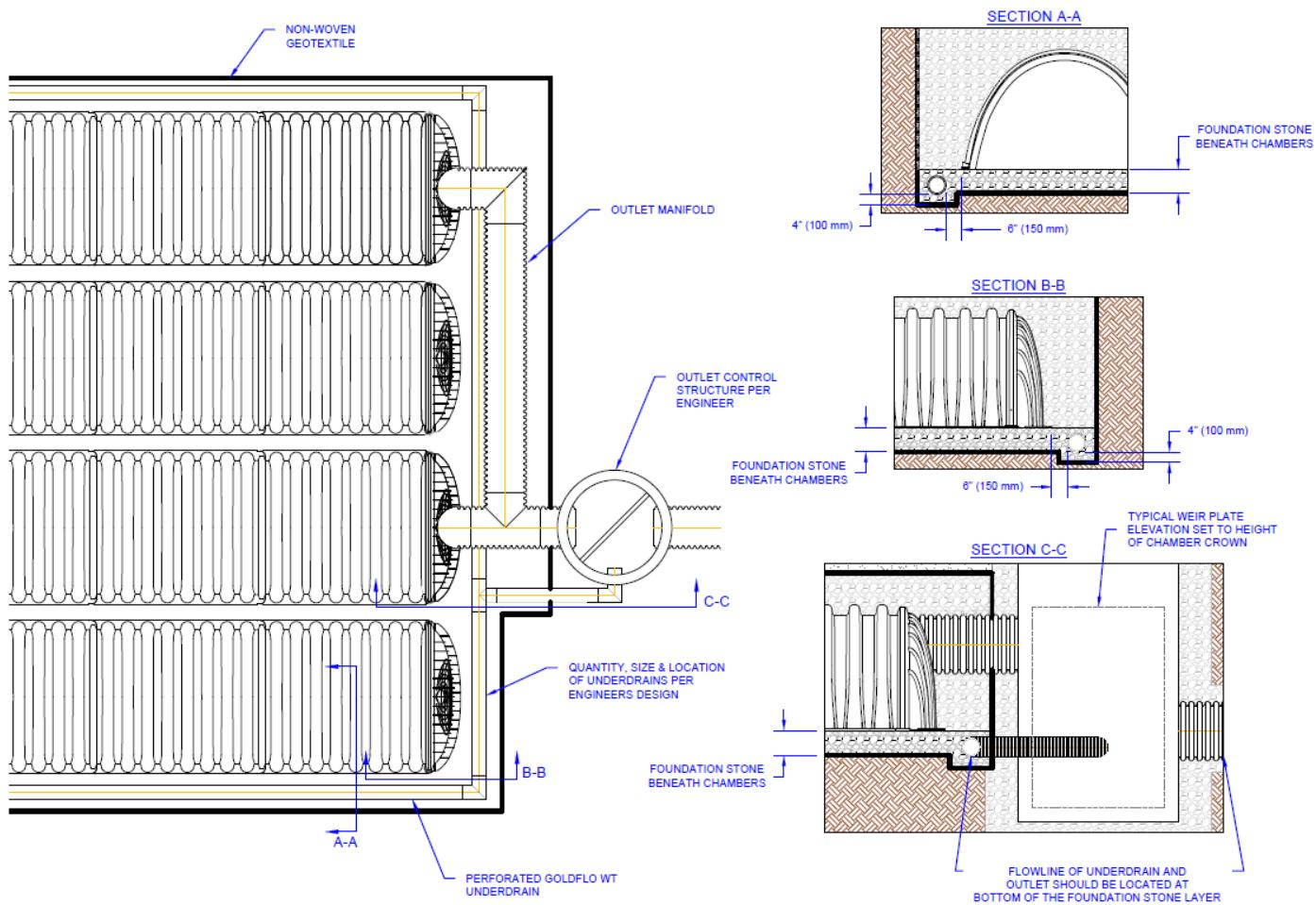
Figure 14 – Optional Underdrain Outlet
