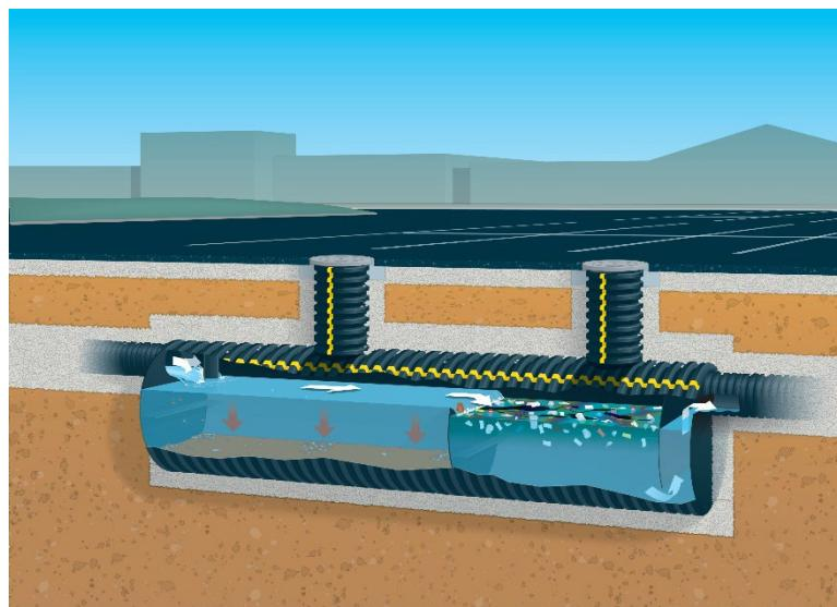
Figure 9 - Prinsco Stormwater Quality Unit (SWQU)
