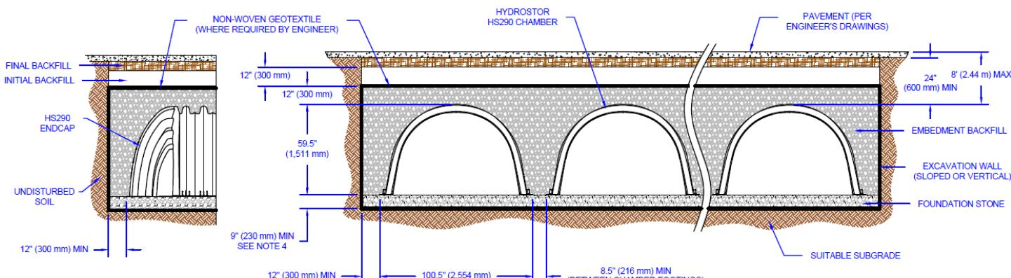
Figure 18 – HS290 Structural Cross Section Detail
