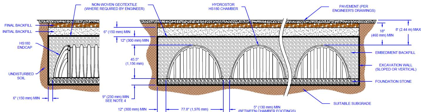
Figure 17 – HS180 Structural Cross Section Detail
