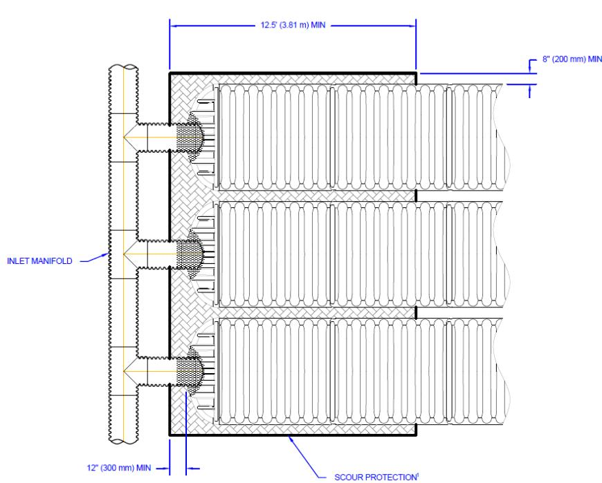
**Figure 13 - Inlet Scour Protection**
