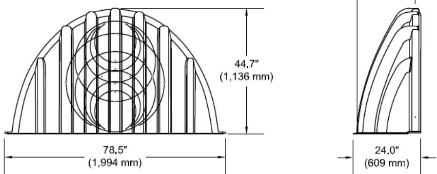
Figure 1 - HydroStor HS180 Chamber & End Caps
