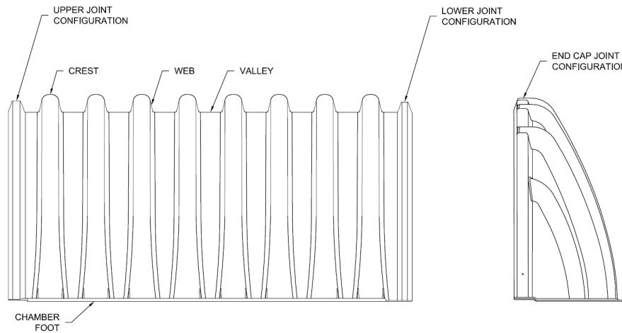
Figure 3 - Chamber and End Cap Components
