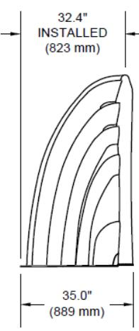
Figure 2 - HydroStor HS290 Chamber & End Caps
