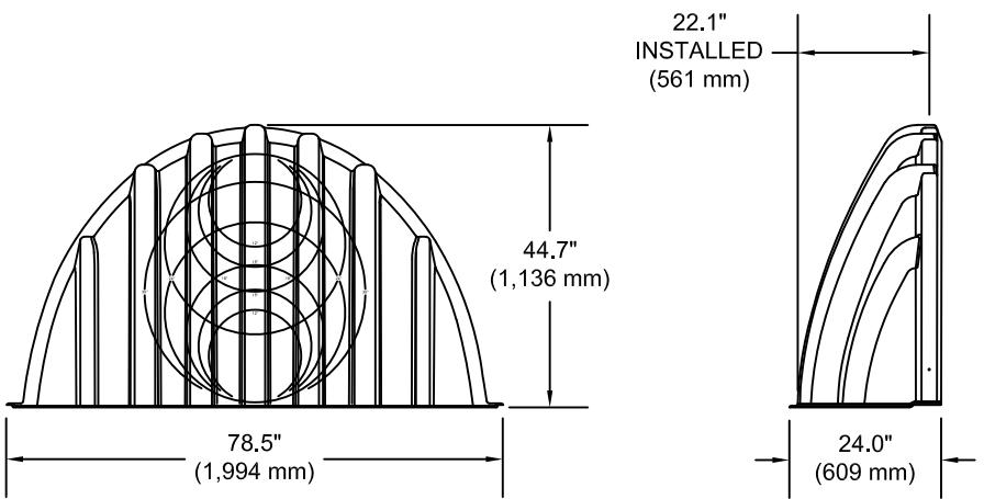
\*ASSUMES 12" (300 mm) STONE ABOVE CHAMBERS/END CAPS, 9" (230 mm) OF STONE FOR FOUNDATION STONE, 5" (130 mm) OF STONE BETWEEN CHAMBERS/END CAPS, 6" (150 mm) OF STONE PERIMETER IN FRONT OF END CAPS AND 40% STONE POROSITY.
