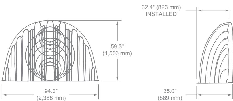
HydroStor® chambers and end caps are engineered to meet or exceed **ASTM F2418** product standards and **ASTM F2787** design standards, as well as **AASHTO H20** live-load and **HL-93** design-load requirements.
